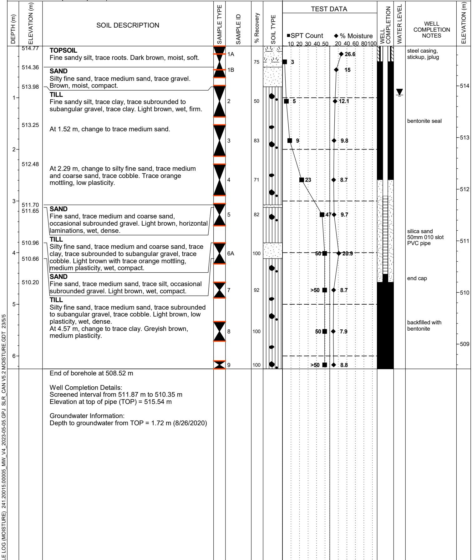
REHO DRILLING METHOD: Hollow Stem Auger Drilling
