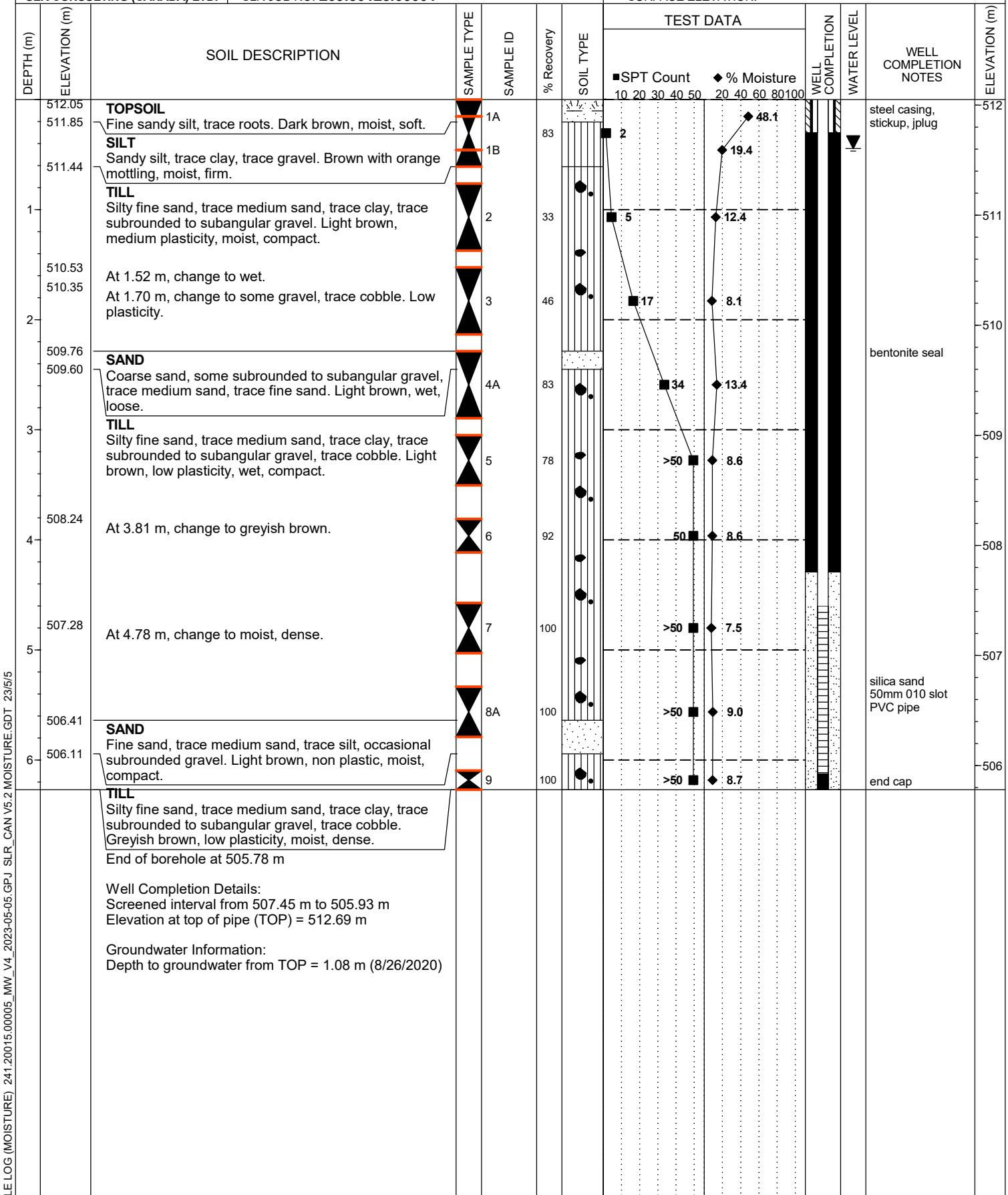
REHO DRILLING METHOD: Hollow Stem Auger Drilling
