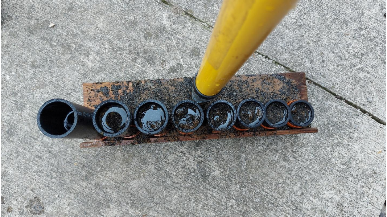
Figure 13: Backwash #2 media expansion result for filter #1 showing media in seven of eight tubes filled with media.
