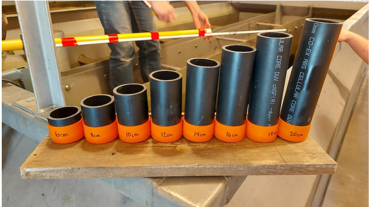
Figure 11: Filter Media Expansion Measurement Tool. In the background: the rod used measure media depth
