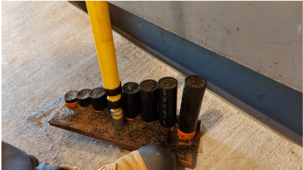
Figure 12: Backwash #1 media expansion results for filter #2. All tubes were filled with filter media
